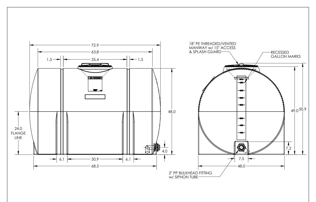
\*ALL EXTERNAL PIPING MUST BE INDEPENDENTLY SUPPORTED. \*ONLY BASE FITTINGS TO BE LEFT INSTALLED AT TIME OF SHIPMENT PER SII PROCEDURE. ALL DIMENSIONS ARE IN INCHES, NOMINAL, & SUBJECT TO CHANGE WITHOUT NOTICE. ALL DIMENSIONS ON ROTATIONAL MOLDED PARTS ARE SUBJECT TO A  $\pm$  3% TOLERANCE.
