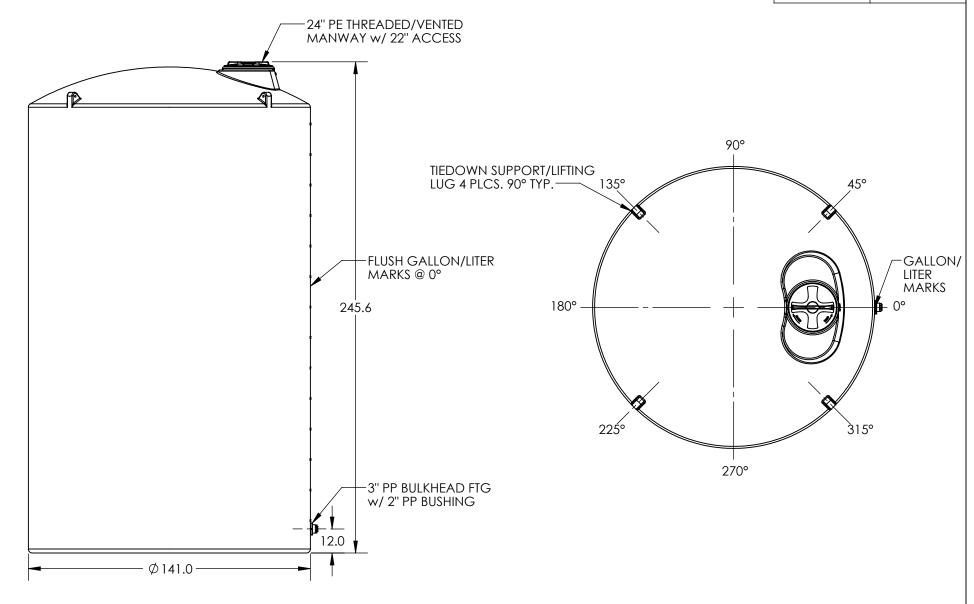
\*ALL EXTERNAL PIPING MUST BE INDEPENDENTLY SUPPORTED. \*ONLY BASE FITTINGS TO BE LEFT INSTALLED AT TIME OF SHIPMENT PER SII PROCEDURE. ALL DIMENSIONS ARE IN INCHES, NOMINAL, & SUBJECT TO CHANGE WITHOUT NOTICE. ALL DIMENSIONS ON ROTATIONAL MOLDED PARTS ARE SUBJECT TO A  $\pm$  3% TOLERANCE.
