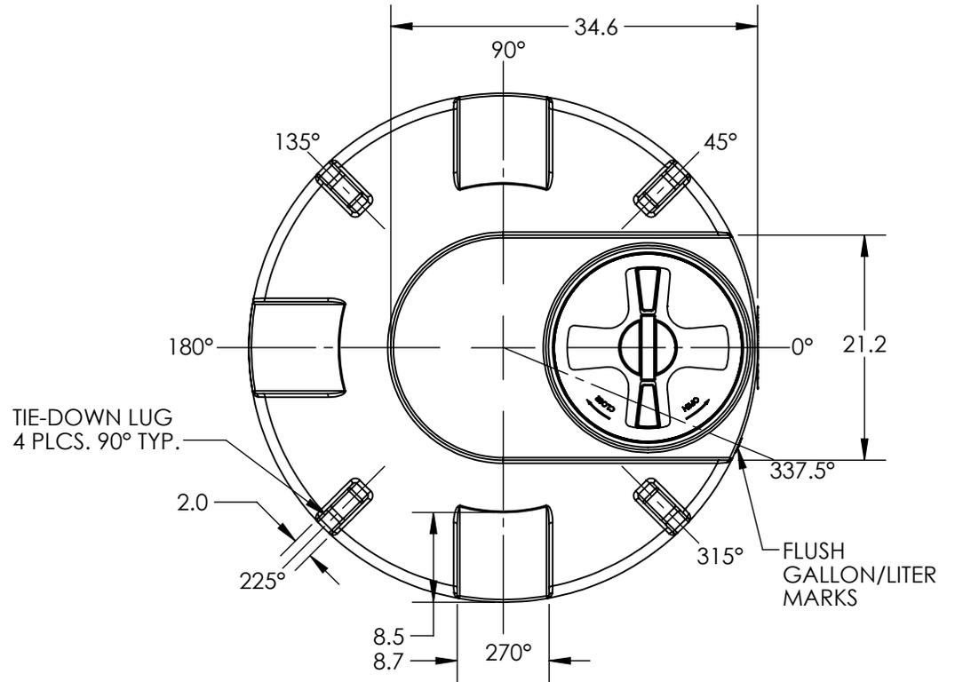
GALLONAGE MARKS CAN BE REMOVED FOR FITTING PLACEMENT AS NEEDED.
