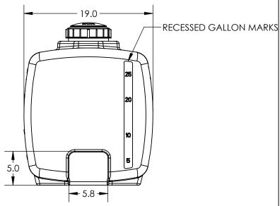
\*ALL EXTERNAL PIPING MUST BE INDEPENDENTLY SUPPORTED. \*ONLY BASE FITTINGS TO BE LEFT INSTALLED AT TIME OF SHIPMENT PER SII PROCEDURE. ALL DIMENSIONS ARE IN INCHES, NOMINAL, & SUBJECT TO CHANGE WITHOUT NOTICE. ALL DIMENSIONS ON ROTATIONAL MOLDED PARTS ARE SUBJECT TO A  $\pm$  3% TOLERANCE.
