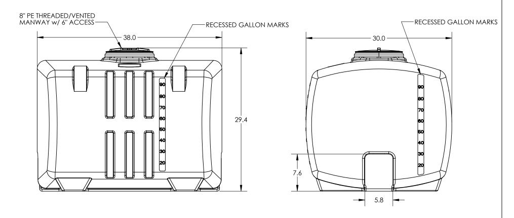
\*ALL EXTERNAL PIPING MUST BE INDEPENDENTLY SUPPORTED. \*ONLY BASE FITTINGS TO BE LEFT INSTALLED AT TIME OF SHIPMENT PER SII PROCEDURE. ALL DIMENSIONS ARE IN INCHES, NOMINAL, & SUBJECT TO CHANGE WITHOUT NOTICE. ALL DIMENSIONS ON ROTATIONAL MOLDED PARTS ARE SUBJECT TO A  $\pm$  3% TOLERANCE.
