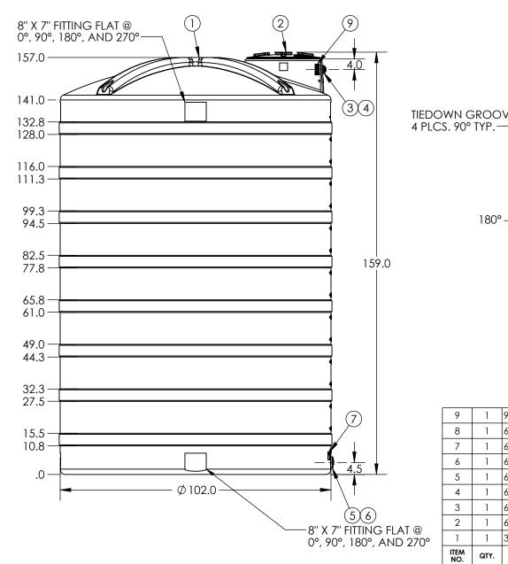
\*FITTINGS ARE CENTERED IN BOTTOM FITTING FLATS & FITTING HEIGHTS MAY VARY. \*ALL EXTERNAL PIPING MUST BE INDEPENDENTLY SUPPORTED. \*ONLY BASE FITTINGS TO BE LEFT INSTALLED AT TIME OF SHIPMENT PER SII PROCEDURE. ALL DIMENSIONS ARE IN INCHES, NOMINAL, & SUBJECT TO CHANGE WITHOUT NOTICE. ALL DIMENSIONS ON ROTATIONAL MOLDED PARTS ARE SUBJECT TO A  $\pm$  3% TOLERANCE.
