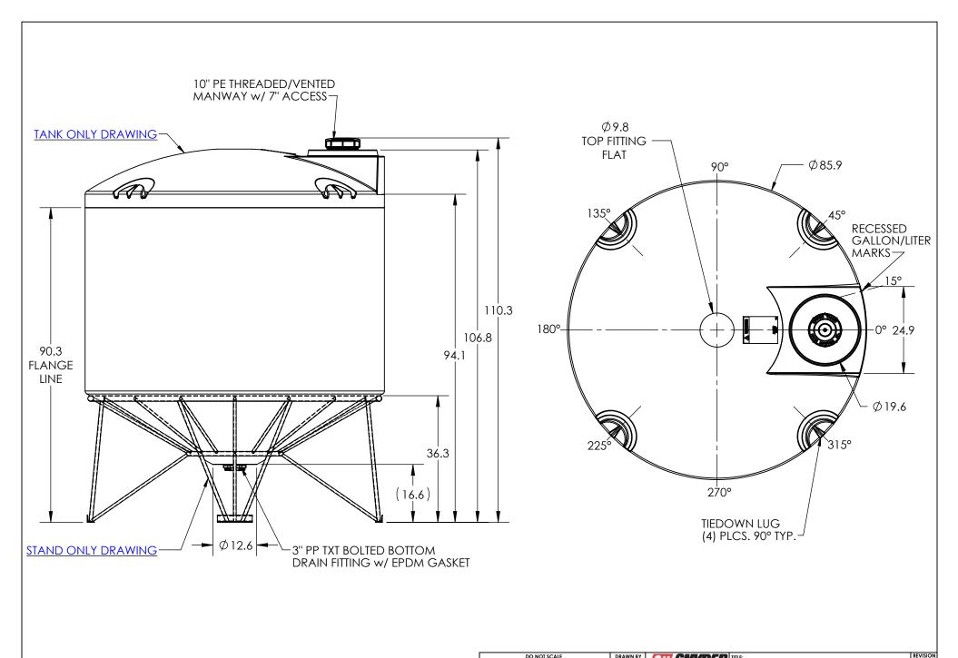
\*ALL EXTERNAL PIPING MUST BE INDEPENDENTLY SUPPORTED. \*ONLY BASE FITTINGS TO BE LEFT INSTALLED AT TIME OF SHIPMENT PER SII PROCEDURE. ALL DIMENSIONS ARE IN INCHES, NOMINAL, & SUBJECT TO CHANGE WITHOUT NOTICE. ALL DIMENSIONS ON ROTATIONAL MOLDED PARTS ARE SUBJECT TO A  $\pm$  3% TOLERANCE.
