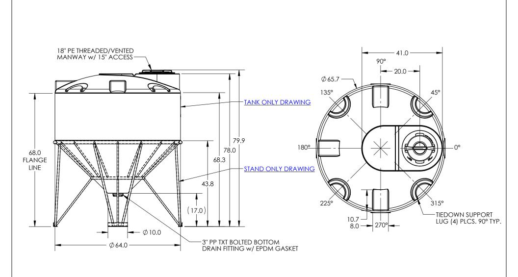
\*ALL EXTERNAL PIPING MUST BE INDEPENDENTLY SUPPORTED. \*ONLY BASE FITTINGS TO BE LEFT INSTALLED AT TIME OF SHIPMENT PER SII PROCEDURE. ALL DIMENSIONS ARE IN INCHES, NOMINAL, & SUBJECT TO CHANGE WITHOUT NOTICE. ALL DIMENSIONS ON ROTATIONAL MOLDED PARTS ARE SUBJECT TO A  $\pm$  3% TOLERANCE.
