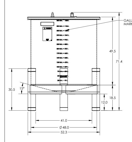
\*ALL EXTERNAL PIPING MUST BE INDEPENDENTLY SUPPORTED. \*ONLY BASE FITTINGS TO BE LEFT INSTALLED AT TIME OF SHIPMENT PER SII PROCEDURE. \*Consult Snyder's Guidelines for Use and Installation prior to delivery.
