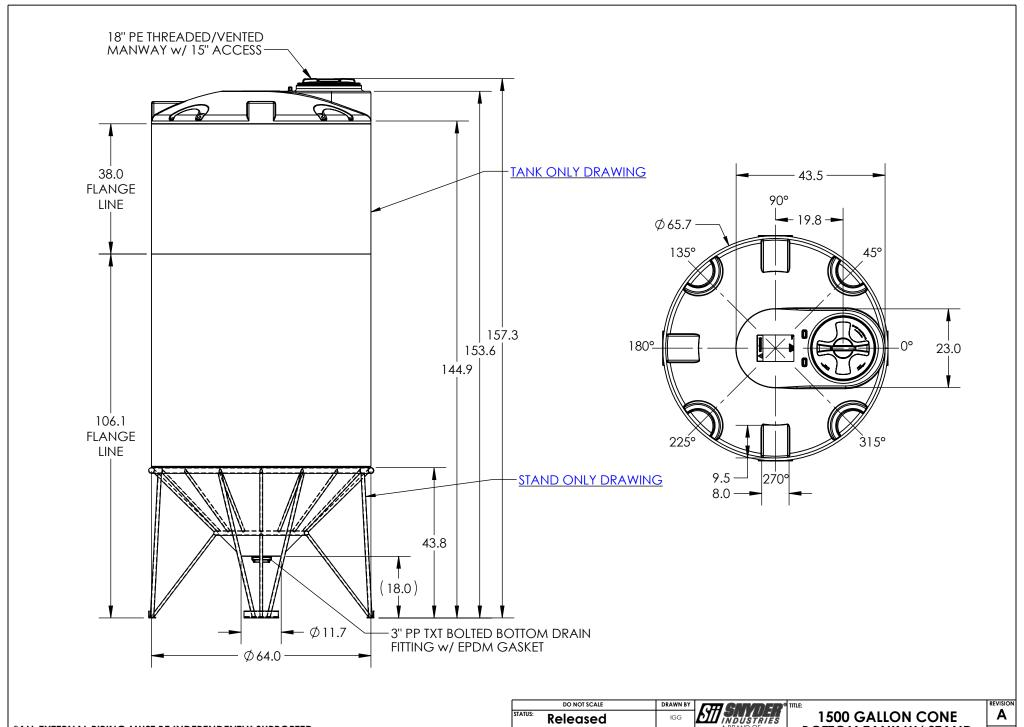
\*ALL EXTERNAL PIPING MUST BE INDEPENDENTLY SUPPORTED. \*ONLY BASE FITTINGS TO BE LEFT INSTALLED AT TIME OF SHIPMENT PER SII PROCEDURE. ALL DIMENSIONS ARE IN INCHES, NOMINAL, & SUBJECT TO CHANGE WITHOUT NOTICE. ALL DIMENSIONS ON ROTATIONAL MOLDED PARTS ARE SUBJECT TO A  $\pm$  3% TOLERANCE.
